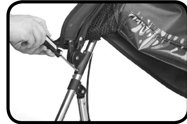
1 Using a phillips head screwdriver, screw brackets to Push Chair frame.
